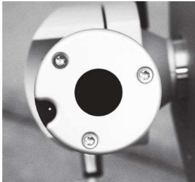
This is an innovative ALL-IN-ONE solar monitoring system with integrated pyrheliometer, shaded pyranometer, digital data processing, GPS receiver and data logger. It measures DNI from the sun and DHI from the sky and, knowing the sun position, calculates GHI that matches secondary standard value. From the DNI measurements sunshine duration is calculated much more accurately than any sunshine duration sensor on the market.
